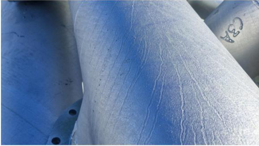
Close up of "fishboning" on abrasive blasted and hot-dip galvanised pipes.
